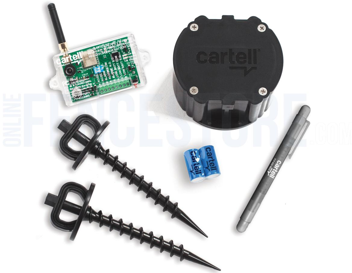
CW-SYS is a wireless system that connects to electric gate operators. Add wireless vehicle detection to any electric gate operator for free exit, whether residential or commercial. Not appropriate for ALL solar gates. Check technical specifications due to 25mA standby current draw from Integrator. Install sensor in the driveway, beside the driveway, or on a post adjacent to the drive.
