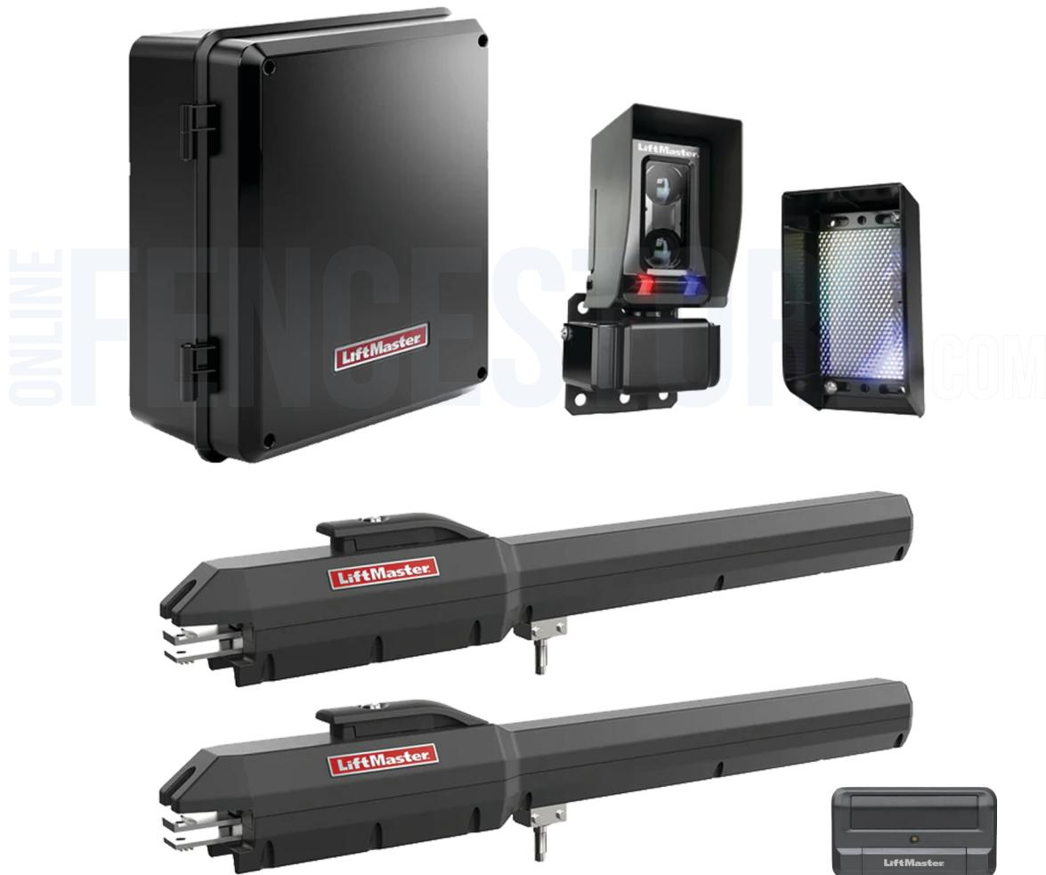
Includes: (1) 811LMX-MC Single Button Programmable Remote, (1) LA500DCS Secondary Actuator Arm, (1) LA500UL Actuator, LMRRUL, LA500CONTUL Standard 24VDC Control Box, (2) 7Ah Batteries, Duty Rating 300 Cycles per day, Power 120V/230 Single Phase, Accessory Power 24VDC 500mA output, UL Usage Classification I, II, III, and IV
