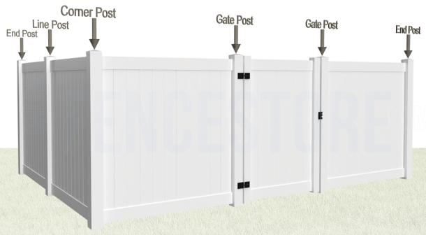
Line Posts join fence panels in a straight line. End Posts end a fence line. Corner Posts connect fence panels together at a 90 degree angle. Gate Posts end a fence line and allows the opening for a gate. Vinyl gate posts also include an internal metal I-beam to provide stability for a swinging gate.
