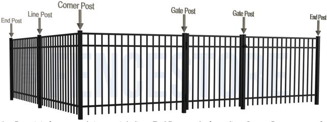
Line Posts join fence panels in a straight line. End Posts end a fence line. Corner Posts connect fence panels together at a 90 degree angle. Gate Posts end a fence line and allows the opening for a gate. Gate posts are thicker than the rest of the posts to provide stability for a swinging gate.
